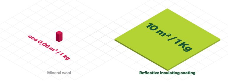
(Mineral wool 150 mm thick, 30 kg/m3, 17.7 kg whole pack, pack yield 1.2 m²) (ABAMAL, 5 I - 2.7 kg, packing capacity 20 m²)
